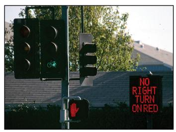
Traffic signal with pedestrian countdown signal and restricts rightturns on red
