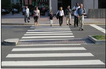
A median nose reduces the exposure time experienced by a pedestrian in the intersection
