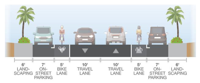
The street cross section modification doesn't have to be expensive. It is possible, for example, to use plastic or rubber pre-fabricated curbing that attaches to the street to designate the new curb instead of poured concrete as shown below.
